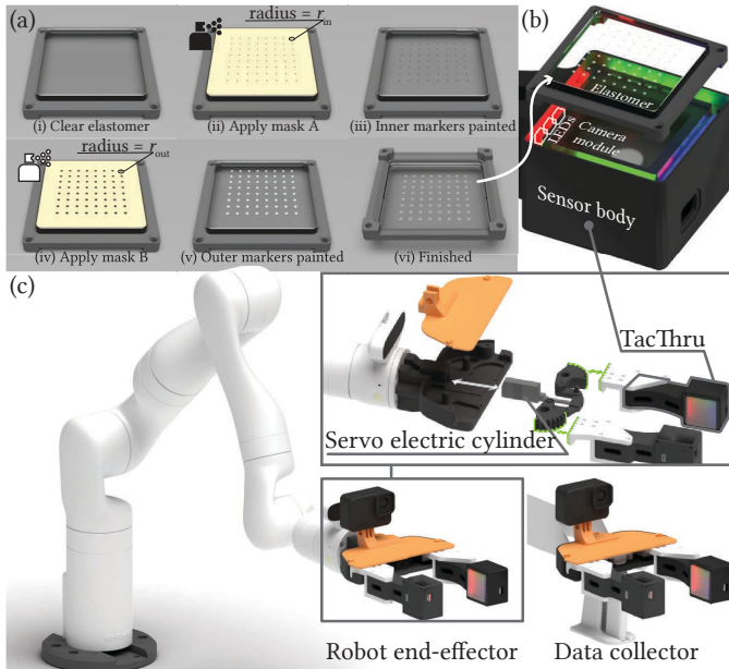
Fig. 2: TacThru’s fabrication and integration in TacThru-UMI. (a) The keyline markers are fabricated by sequentially spraying inner (black) and outer (white) markers on a transparent elastomer. (b-c) TacThru-UMI includes a robot end-effector (left) and a data collector (middle) with identical body and TacThru fingers. The end-effector’s fingers are actuated by a servo electric cylinder (right).
