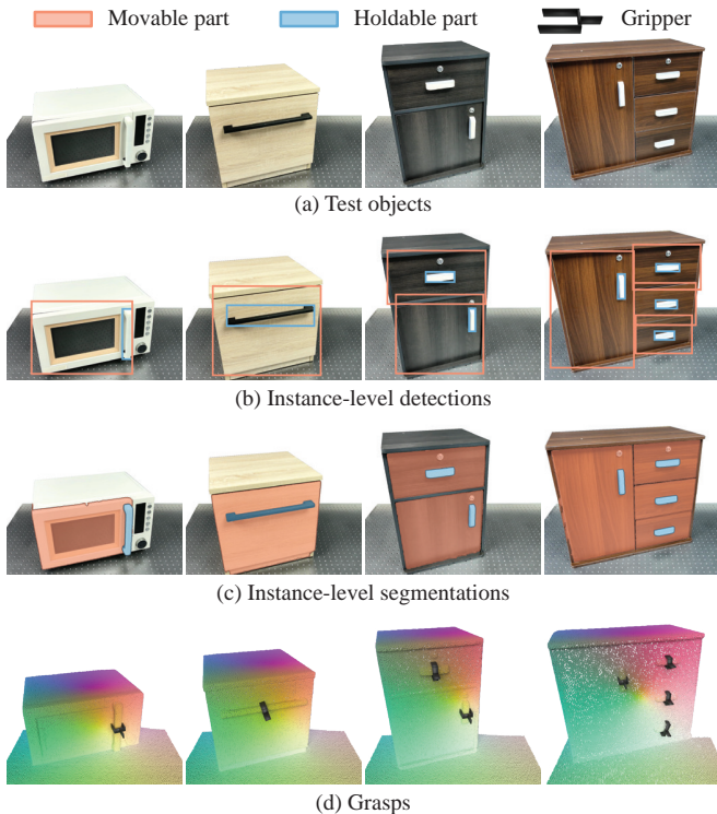
Fig. 4: Real-world articulated objects and processing pipeline. (a) We evaluate Vi-TacMan on real-world objects spanning diverse configurations: prismatic to revolute joints, and single-part to multi-part structures. (b) Our trained detector reliably identifies movable and holdable parts, even in complex multi-part cases. (c) These detections provide prompts for the segmentation model, enabling fine-grained part segmentation. (d) Based on segmented parts, suitable grasps are generated at grasping points g . These results provide the necessary information for inferring interaction directions.
