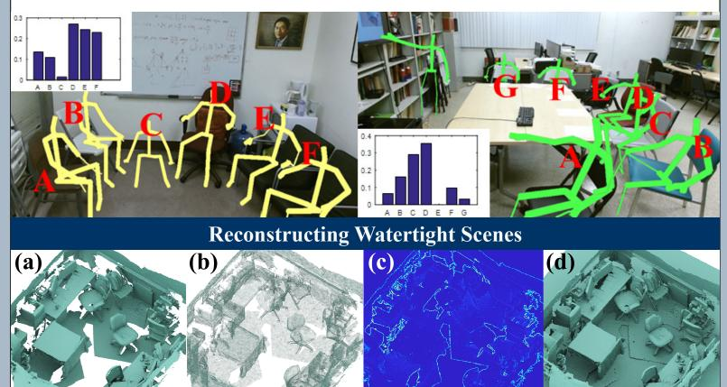
From a reconstructed 3D indoor scene (a), we uniformly sample vertices in the input mesh with Poisson disk sampling (b), then convert them into a watertight mesh (d) with well-defined interior and exterior regions. Differences (c) between the input mesh and the converted watertight mesh.
