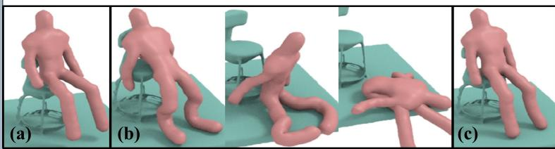
Given an initial human pose in a 3D scene subject to gravity (a), without adequate damping (b) the human body is too energetic and produces unnaturally bouncy motion. With proper damping, the simulation converges to a physically stable rest pose (c) in a small number of timesteps.
