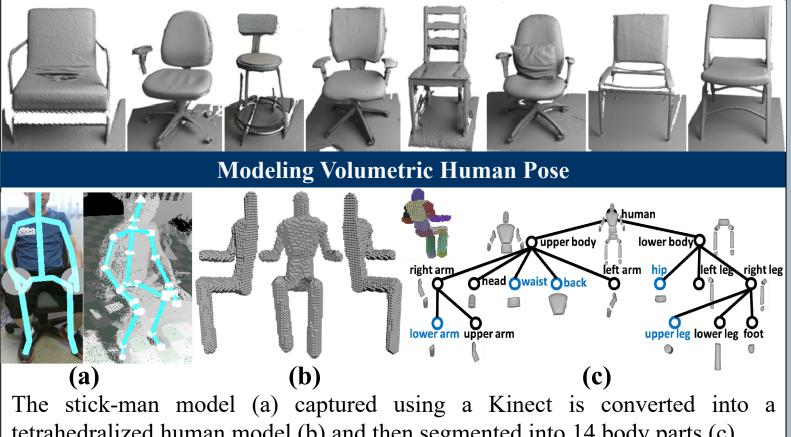
tetrahedralized human model (b) and then segmented into 14 body parts (c).
