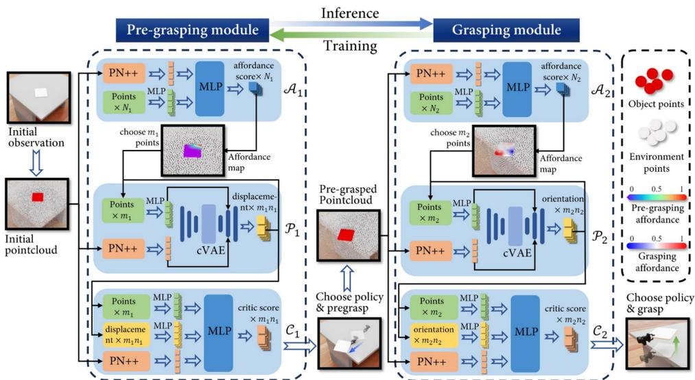
Pre-grasping and grasping are managed by the pre-grasping module and the grasping module, respectively. Within each module, three specialized neural networks are employed: an affordance network  $\mathcal{A}$ , a proposal network  $\mathcal{P}$ , and a critic network  $\mathcal{C}$ .
