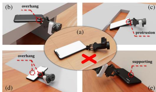
But by repositioning the object before grasping, and leveraging environmental features like Edge, Slot, Slope, Wall, the object becomes graspable.
